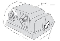
2 Check that there is oil in the transmission's oil tank.
