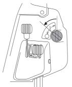
3 When the Rider is at a standstill, press down the parking brake and push in the locking button.
