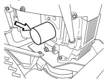
Lightly lubricate the rubber seal on the new oil filter using new oil. Fit the oil filter by turning clockwise. Turn by hand until the rubber seal is seated. Now tighten a further half turn.
