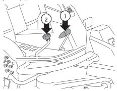
3 Select the required cutting height (1-7) with the cutting height lever.
