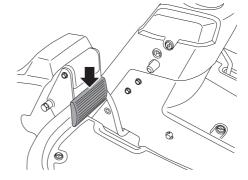
2 Carefully press down one of the pedals until the required speed is obtained. Pedal (1) is used to drive forwards, and pedal (2) to drive backwards.
