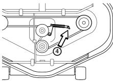
Simply reverse the procedure to fit the new belt.
