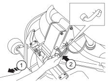
10 Grasp the front edge of the cutting unit, pull out and raise into the service position.
