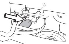
3 Insert the bolt and secure it with a locking pin.
