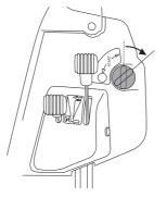
6 When the engine starts release the ignition key immediately back to neutral position.
