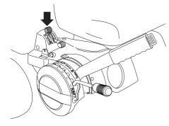
To increase or reduce the engine speed the control is moved forwards or backwards.
