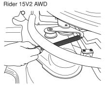
6 Place a foot on the front edge of the cutting unit near the wheel and raise the front edge of the unit to make it easier to remove the lift strut.
