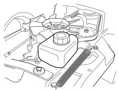
**Rider 15V2** Fill if necessary with engine oil SAE 10W/30 (class SF–CC).
