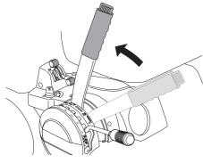
If the lock button is pressed in and the lever is moved forwards the unit will be lowered and the blades will automatically start to rotate (mowing position).
