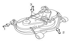
1 Place the Rider on a flat surface and apply the parking brake. Check that the lever for setting the cutting height is in the lowest position.
