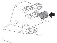
8 Let the engine run at moderate speed or half throttle for 3-5 minutes before subjecting it to heavy load.
