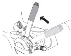
Rider 15V2 AWD. The engine can not be started if the parking brake is not pressed down.
