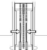
3 If necessary, the wires can be adjusted by tightening the adjuster nuts on each side of the steering collar. Do not over tighten the cables; they should only be drawn in towards the steering collar.
