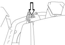
· Replace the pump on the console.
