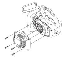
• Pull out the cord approx. 30 cm and hook it into the notch in the rim of the pulley. Release the recoil spring by letting the pulley rotate slowly backwards.
