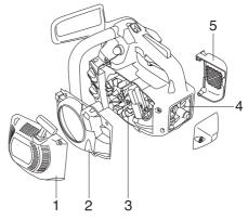
Clean the cooling system with a brush once a week, more often in demanding conditions. A dirty or blocked cooling system results in the machine overheating which causes damage to the piston and cylinder.
