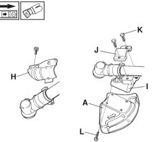
Remove the mounting plate (H). Fit the adapter (I) and bracket (J) with the two screws (K) as shown. Fit the blade guard (A) to the adapter using the 4 screws (L) as shown.
