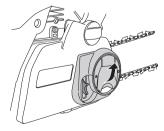
• Turn the knob anti clockwise to loosen the bar cover.
