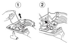
Undo the bolt in the centre of the pulley and remove the drive disc (A), drive disc spring (B) and the pulley (C). Insert and secure a new starter cord in the starter pulley. Wind approx. 3 turns of the starter cord on the starter pulley. Fit the starter pulley so that the end of the recoil spring (D) hooks into the starter pulley. Now assemble the drive disc spring, drive disc and the bolt in the centre of the pulley. Carry the starter cord
