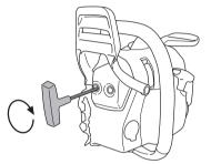
Some mufflers are equipped with a special spark arrestor mesh. If your machine has this type of muffler, you should clean the mesh at least once a week. This is best done with a wire brush. A blocked mesh will cause the engine to overheat and may lead to serious damage.
