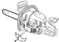
CAUTION! If the special winterising kit has been fitted or any measures have been taken to increase the temperature these changes must be reversed before the machine is used in normal temperature conditions. Otherwise there is a risk of overheating, resulting in severe damage to the engine.
