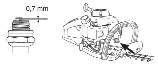
**CAUTION!** Always use the recommended spark plug type! Use of the wrong spark plug can damage the piston/cylinder. Check that the spark plug is fitted with a suppressor.
