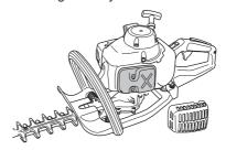
Some mufflers are equipped with a special spark arrestor mesh. If your machine has this type of muffler, you should clean the mesh at least once a week. This is best done with a wire brush.
