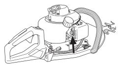
Choke: Set the choke control in the choke position.
