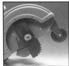
6. Slowly lift the handle to lower the blade, finding the edge of the paved surface and start edging. Then move tool forward slowly along edge of paved surface, keeping the edge guide pressed lightly against the pavement edge.
