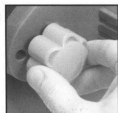
Raise or lower the arm to the desired position, and then pull the height adjusting knob outwards. Rotate the knob in a clockwise direction until all of the slack is taken out of the assy. Check to ensure the
