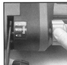
front wheel arm has located into one of the pre allocated positions and the head of the bolt securing the front wheel arm is sitting flat on the surface of the wheel arm.
