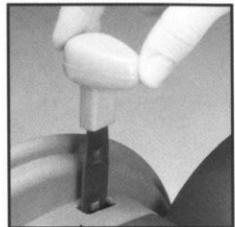
The Edge Guide Control Knob should be returned to the upright position to lock the Guide in the down position.
