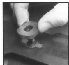
To re assemble with the a new blade fit the inner flange on to the spindle, fit the replacement blade and secure the outer flange on to the spindle and blade.
